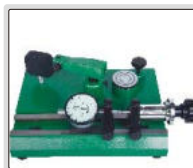
inspect accuracy of dial indicators (range 0-25mm)
