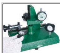
test force of dial indicators
